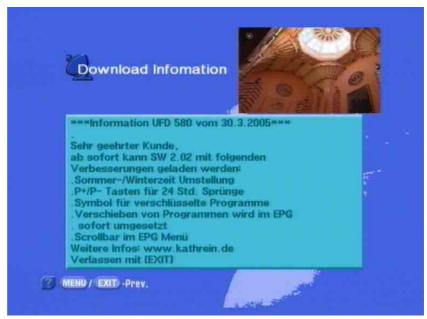
Once the update is complete, the receiver is re-initialised and starts operation again. In case of an error or no signal, the message "**Download failed**" appears.
